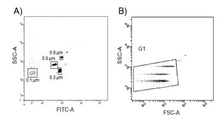
A) Gate limits were established before analyses using the Megamix-Plus FSC beads for cytometer settings in microparticle analysis (BioCytex, Marseille, France). According to Megamix-Plus FSC beads signal, the lower limit of quantification is >0.1µm, as beads of 0.1µm were negative for FITC signal. B) Gate limits for microparticle quantification (G1) were set according to beads signal.
