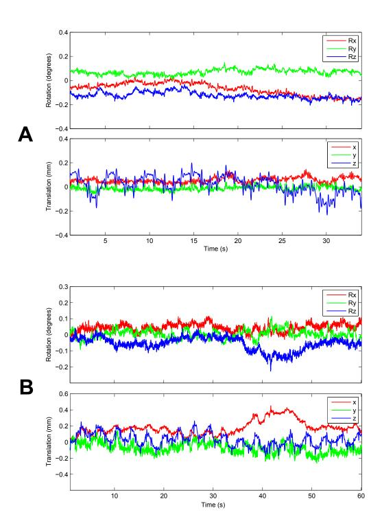
**Fig. S2.** Tracking data from (A) the 1.5 T and (B) the 3 T experiments. In these examples, the MPT marker was attached directly to the forehead of the subject; this differs from the results obtained at 7 T, and shown in Fig. 5, where a mouthpiece was used. With both marker attachment methods (and for all three scanners and subjects), the ballistocardiogram is visible in the z direction. In the examples shown here, respiratory motion is also clearly visible.
