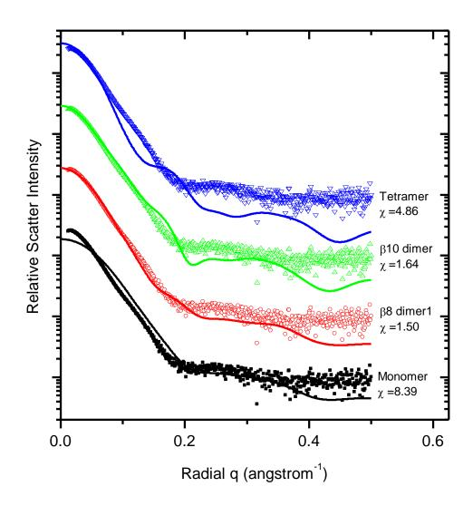
**Figure S6: X-Ray scattering of** *At-***DHDPR2**. Data was collected and compared to the scattering calculated using CRYSOL for the monomer,  $\beta$ -10 dimer,  $\beta$ -8 dimer, and tetramer of *Ec-*DHDPR.
