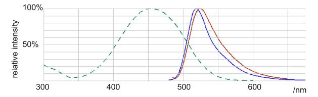
**Figure S4**: UV/VIS spectra of the quencher DABCYL and the fluorophore FITC. Absorbance spectrum of DABCYL (green dashed line), emission spectra of FITC as an fluorescein antibody conjugate (blue line) and as a fluorescein-dextran conjugate (red line), both at pH 8.0; adapted from the online Fluorescence Spectra Viewer (http://probes.invitrogen.com/servlets/spectra/) with kind permission from Dr. Iain Johnson, Invitrogen Corporation, Molecular Probes.
