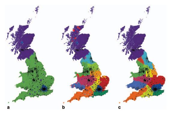
**Figure 2. Defining regions through the spectral modularity optimization of telecommunications networks.** a - even with just three regions we obtain a total modularity of 0.31, indicating a fairly good network partitioning. b - the final partitioning of Great Britain yields a modularity of 0.58. c - further fine tuning according to the process suggested by Newman [16] increases the modularity to 0.60. doi:10.1371/journal.pone.0014248.g002
