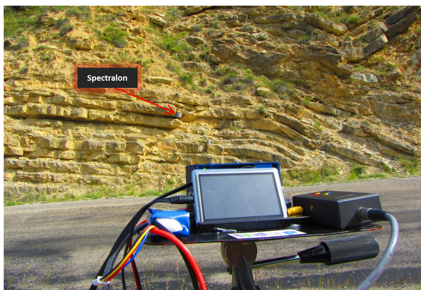
Fig 5. Positioning of the multispectral camera with respect to a rock formation including the Spectralon placed on the wall of the rock.
