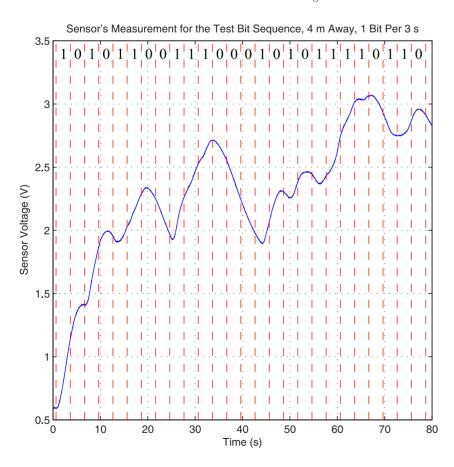
**Figure 13. Received signal when a 26 bit test sequence is transmitted.** Sensor reading for the 26 bit test sequence "1010110011100101111010" transmitted 4 meters away at the rate of one bit per 3 seconds. The dashed red lines represent the start and the end of each bit. Honeywell fan is used to create the flow for this figure. doi:10.1371/journal.pone.0082935.g013
