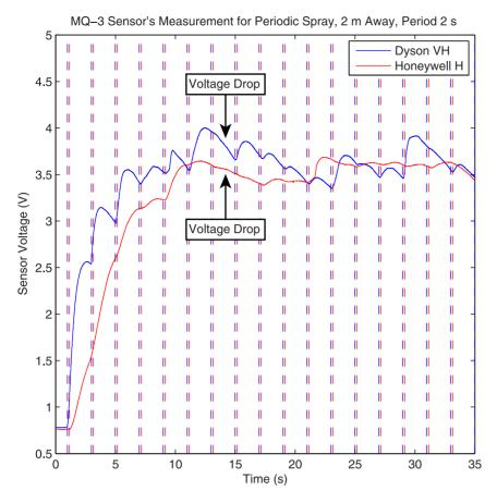
**Figure 12. System response to a periodic spray.** The dashed lines are 2 seconds apart and show each period. The arrows show the location where the sensor voltage decreases instead of increasing. The spray duration is 100 ms, and the separation distance is 2 m. doi:10.1371/journal.pone.0082935.q012
