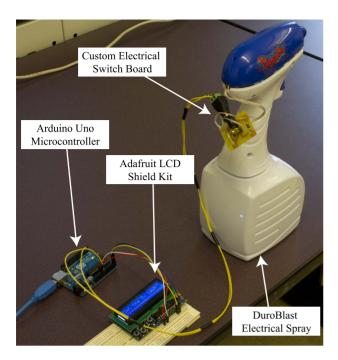
**Figure 2. The transmitter components.** doi:10.1371/journal.pone.0082935.g002
