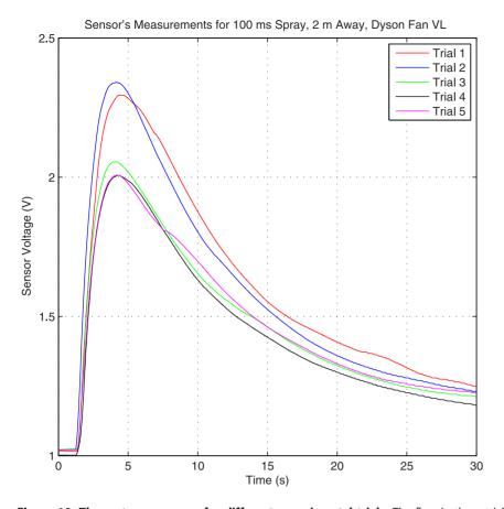
**Figure 10. The system response for different experimental trials.** The flow in these trials is generated using the Dyson fan on very low setting. The spray duration is 100 ms, and the separation distance is 2 m. doi:10.1371/journal.pone.0082935.g010
