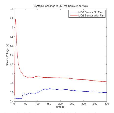
**Figure 5. Diffusion based propagation versus flow based propagation.** The system response to a 250 ms spray 2 meters away for diffusion based propagation (blue), and flow based propagation (red). doi:10.1371/journal.pone.0082935.g005
