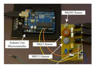
Figure 3. The receiver components. doi:10.1371/journal.pone.0082935.g003
