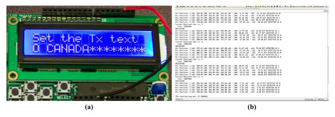
**Figure 14. Transmitted and received text message.** Pictures from a communication session: (a) the text entered at the transmitter (b) the text received at the receiver. doi:10.1371/journal.pone.0082935.g014
