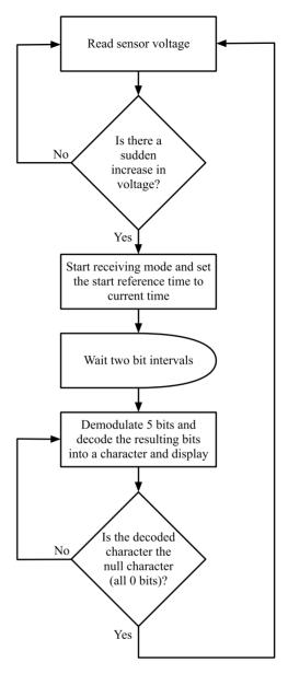
Figure 7. Flowchart representation of the algorithm that controls the receiver.
