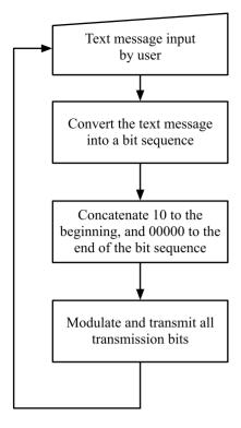
Figure 6. Flowchart representation of the algorithm that controls the transmitter.
