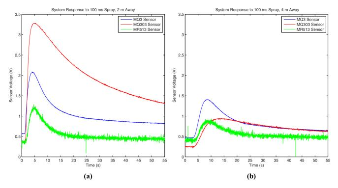
**Figure 8. Comparing the three sensors.** The system response to a short spray of 100 ms for all three sensors at (a) 2 m separation, and (b) 4 m separation between the transmitter and the receiver. doi:10.1371/journal.pone.0082935.g008
