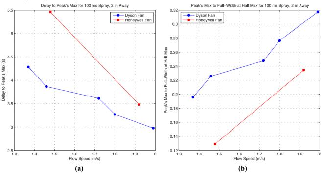
**Figure 11. Analysis of the system response for different flows.** The delay to peak's maximum is used as one performance metric (a), and the peak's maximum to full width at half max is used as a second performance metric (b). The results from 10 different trials are averaged to create each point. The spray duration is 100 ms, and the separation distance is 2 m. doi:10.1371/journal.pone.0082935.g011
