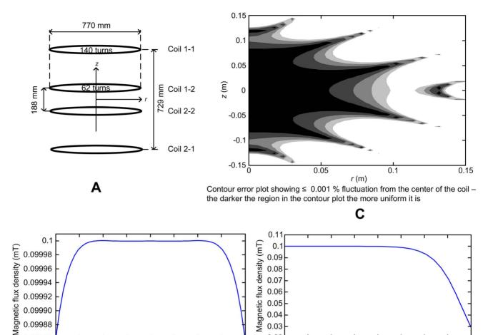
Figure 4. The Lee-Whiting coil. (A) Coil design, (B) (i) magnetic flux distribution in the z-direction, (ii) magnetic flux density distribution in the rdirection, and (C) fluctuation of the magnetic flux density from the center of the coil. doi:10.1371/journal.pone.0081227.g004
