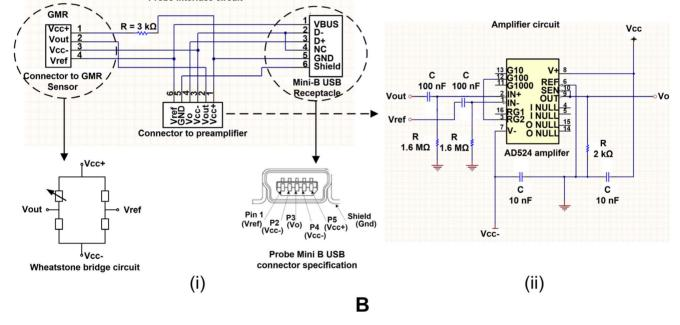
**Figure 3. The giant magnetoresistance probe.** (A) (i) Needle sensor, and (ii) Wheatstone bridge design of the sensors. (B) (i) Probe interface circuit, and (ii) amplifier circuit. (C) Fabricated probe with the USB connector. doi:10.1371/journal.pone.0081227.g003
