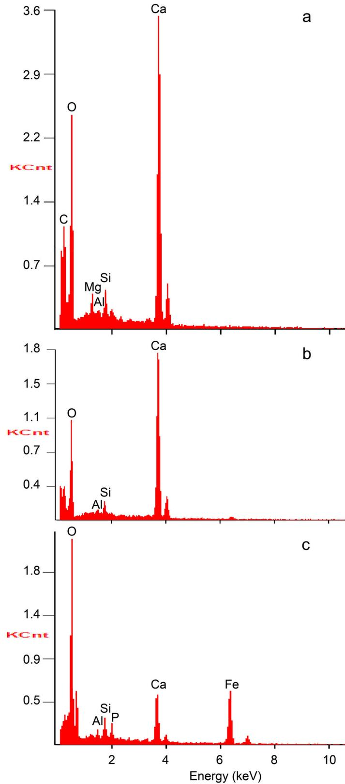
**Figure 8. Results of the Energy Dispersive X-ray analysis performed on the Fumane *Aspa marginata* shell.** a: outer shell surface, b: broken crystals on the edge of the micropit shown in Figure 7d, c: red substance filling the pit (Figure 7c).
