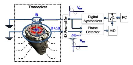
**Figure 1. Schematic of the VEPS Head/coil configuration and a block diagram of the experimental prototype.** The system consists of five modules: digital synthesizer, transceiver, phase detector, data acquisition and data processing. doi:10.1371/journal.pone.0063223.q001
