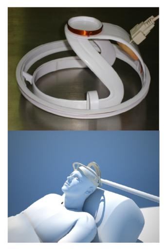
Figure 2. Photographs of the VEPS clinical Head/coil device and an illustration of a patient in a critical care unit wearing the device.
