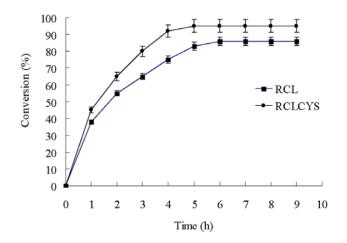
Figure 7. Time course of solvent-free conversion of soy bean oil to fatty acid methyl esters by RCLCYS and RCL at 40°C. doi:10.1371/journal.pone.0046388.g007
