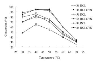
Figure 6. Solvent-free conversion of soy bean oil to fatty acid methyl esters by RCLCYS and RCL at different temperatures. The various curves refer to the conversion of soy bean oil by lipases as a function of temperature at different intervals of reaction time. doi:10.1371/journal.pone.0046388.g006
