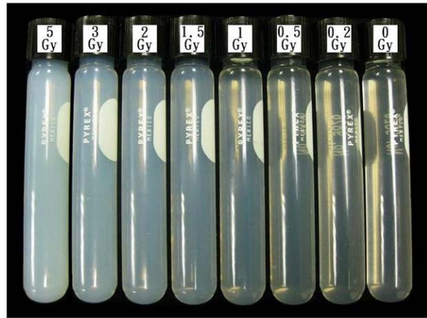
**Figure 1. Glass vials of NIPAM gels irradiated to graded doses.**
