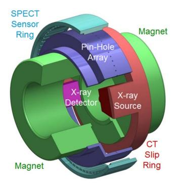
Figure 5. Double-magnetic-donut-based design for omnitomography. The pair of green magnetic rings is arranged similar to that in the Fonar UPRIGHT Multi-Position MRI (http://www.fonar.com/ standup.htm) but with a decreased spatial extent of a homogeneous magnetic background field and thus an increased gantry room for interior CT, interior SPECT, and other modalities. This design is scalable according to preferred sizes of animals or humans. doi:10.1371/journal.pone.0039700.g005
