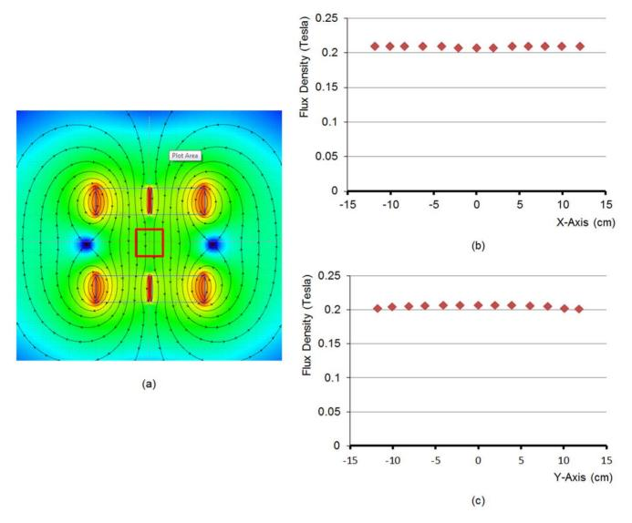
**Figure 4. Generation of a locally homogeneous magnetic field.** (a) The magnetic flux from four permanent blocks. The square area  $(20 \times 20 \text{ cm}^2)$  represents a region of interest (ROI) where the magnetic flux ranges from 0.208 to 0.211Tesla; (b) and (c) the magnetic flux plots along the x- and y-axes respectively. Each magnetic block is of  $40 \times 40 \times 20 \text{ cm}^3$ , with a gap of 2 cm between two parts of each magnetic pole. doi:10.1371/journal.pone.0039700.g004
