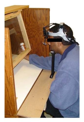
Figure 5. Experimental set up (chin rest, calibrated plane and the head-mounted optics of our ASL 501 eye tracking unit). doi:10.1371/journal.pone.0038819.g005
