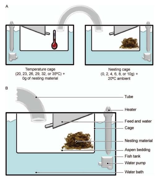
**Figure 1. Titration apparatuses.** (a) Diagram showing the configuration of water baths and cages for testing cage temperature and nesting material preferences. (b) Diagram depicting elements present in water bath and cage setup. The figures are reproduced with permission from Elsevier [5,6] doi:10.1271/journal.page.0022700.c001
