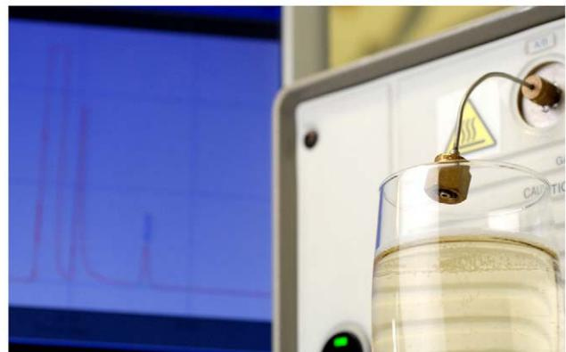
**Figure 2. Gas chromatograph injection valve sampling gases in the headspace above the flute.** Photograph by Gérard Liger-Belair. doi:10.1371/journal.pone.0030628.g002
