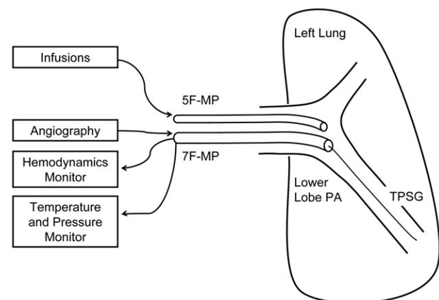
**Figure 1. Experimental setup:** Using femoral vascular access, a 7F multipurpose (MP) guiding catheter was placed in a left lower lobe segmental pulmonary artery (PA). A 5F-MP was placed alongside the 7F-MP and positioned proximal to it. A temperature and pressure sensor guidewire (TPSG) was passed through the 7F-MP and placed within the distal PA.
