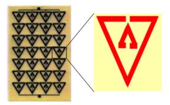
Figure 4. Fabricated TSRRs structure for the SAR measurement. doi:10.1371/journal.pone.0109947.q004
