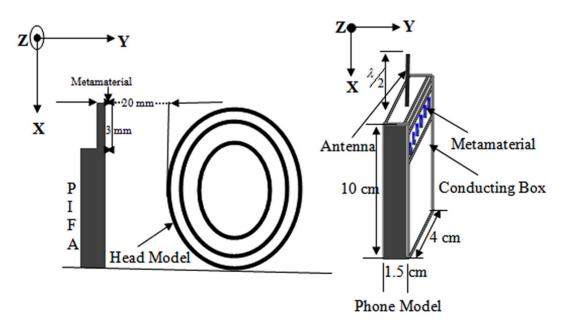
Figure 1. The head and antenna model for SAR calculation. doi:10.1371/journal.pone.0109947.q001
