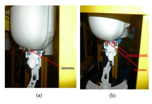
Figure 8. Measurement of the SAR values at the cheek position a) without a metamaterial and b) with a metamaterial doi:10.1371/journal.pone.0109947.g008
