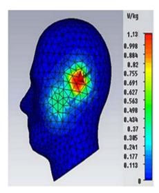
Figure 10. Simulated SAR value of the antenna with the TMMs attachment in the cheek position.
