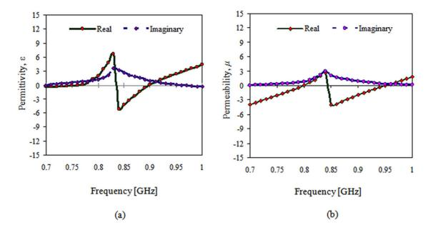
Figure 5. Materials measured at the resonant frequency are double negative: a) negative permittivity and b) negative permeability. doi:10.1371/journal.pone.0109947.g005
