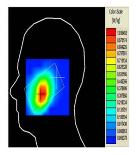
Figure 11. Measured SAR of the antenna with the TMMs attached in the cheek position.
