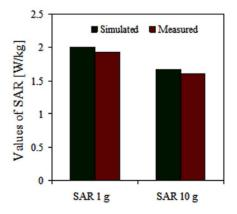
Figure 7. Comparison on SAR simulation and measurement results without the inclusion of TMMs. doi:10.1371/journal.pone.0109947.g007
