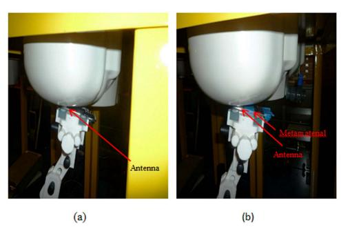
Figure 9. Measurement of the SAR values at the tilt position a) without a metamaterial and b) with a metamaterial. doi:10.1371/journal.pone.0109947.q009
