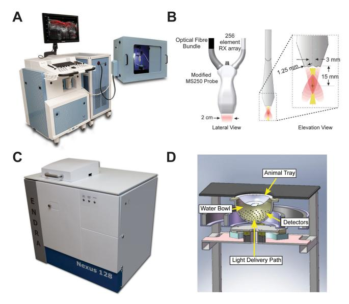
**Figure 2.** Schematics of experimental systems used. (A) The VisualSonics Vevo LAZR uses intersecting planar laser beams (B) for excitation and a linear transducer array for 2D imaging of the resulting ultrasound. (C) The Endra Nexus 128 delivers diffuse laser light and detects the ultrasound using 128 transducers in a helical arrangement (D) for 3D reconstruction. doi: 10.1371/journal.pone.0075533.g002
