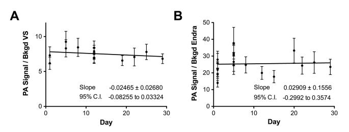
**Figure 5. Reproducibility of photoacoustic imaging measurements over time using the quality control phantom.** Stability of VisualSonics (A) and Endra (B) over time assessed by repeated imaging of phantom P1 at 750 nm. First 30 days shown for clarity, but coefficient of variation values derived out to 4 months shown in Table 2. Abbreviation VS = VisualSonics. doi: 10.1371/journal.pone.0075533.g005
