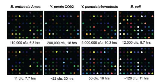
**Figure 3. Color difference maps of** *B. anthracis* **Ames**, *Y. pestis* **CO92**, *Y. pseudotuberculosis*, **and** *E. coli*. Each color represents the difference between the indicator color intensity measured before exposure and the intensity measured at the indicated detection time for each species. For visualization purposes, color difference maps are expanded from 4 to 8 bits per color (RGB range of 0–15 expanded to 0–255) [33]. doi:10.1371/journal.pone.0062726.g003
