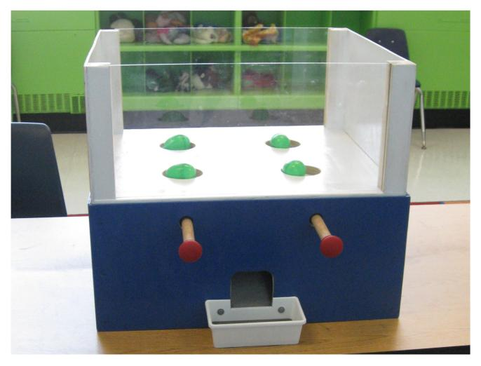
Figure 1. A view of the experimental set-up taken from the actor's side of the apparatus. The actor was able to pull one of the two bars in order to deliver the allocations displayed on the top of the apparatus. Trial pictured is in the visible condition with opaque containers. doi:10.1371/journal.pone.0048292.q001
