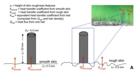
Figure 2. Schematic of our heat-transfer model showing model configuration and various parameters relating to rough and smooth skin (*individual hair in small box in top-right corner is enhanced for illustrative clarity*). doi:10.1371/journal.pone.0047018.g002
