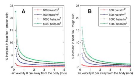
Figure 4. Increase in heat transfer due to hair, reported as a percentage  $h_{hair}/h_{skin} \times 100$ , as a function of ambient wind speed for different hair densities on smooth skin (A), and rough skin (B). The heat transfer increase due to hair on our example elephant – which has a hair density of ~650 hairs/m<sup>2</sup>- is ~10% at low wind speed and decreases as the wind speed increases. doi:10.1371/journal.pone.0047018.g004
