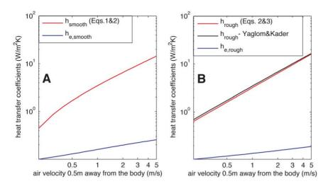
Figure 3. Variation of the different heat transfer coefficients with wind speed for a hair density of 1500 hairs/m<sup>2</sup>. (A) Heat transfer coefficient for bare smooth skin and effective heat transfer coefficient for hair over smooth skin. (B) Same as A, but for rough skin. B also depicts the alternative formulation for  $h_{rough}$  of Yaglom and Kader [18]. doi:10.1371/journal.pone.0047018.g003
