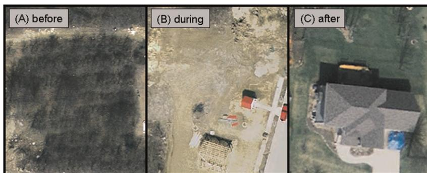
**Figure 1. Aerial photos of research plots representative of each stage of habitat disturbance.** (A) before construction: naturalized apple orchard, (B) during construction: trees and top soil are removed to prepare the ground for construction, (C) after construction: sodded lawn and landscape trees are installed, the house covers majority of the plot.
