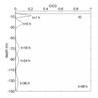
Figure 5. Analytical solution of the distribution of sinking bluefin tuna eggs in the Black Sea over time (0-48h). Particles have been released at time t0 and depth z0=5 m with an initial concentration C<sub>0</sub> and terminal velocity W = 1 mm s<sup>-1</sup>, corresponding to egg density = 1019 kg m<sup>-3</sup>. doi:10.1371/journal.pone.0039998.g005
