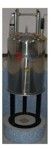
**Figure 1.** Photograph of the diamagnetic levitation apparatus. The apparatus is located in the Key Laboratory for Space Biosciences & Biotechnology of the Northwestern Polytechnical University, China. doi:10.1371/journal.pone.0024697.g001
