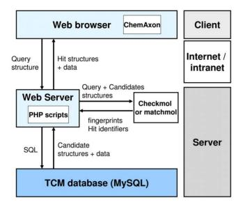
Figure 4. The infrastructure of the TCM database. The design is adapted from Norbert Haider's MoIDB5R. doi:10.1371/journal.pone.0015939.g004
