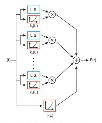
**Figure 5. Schematic view of the adaptive QLV model (Eq. 17).** Blue is used for linear processes, and red is used to indicate nonlinearities. Because the nonlinearity does not precede the linear stage (L.S.), superposition does not hold (unlike the QLV model, Fig. 1B). doi:10.1371/journal.pone.0006480.g005
