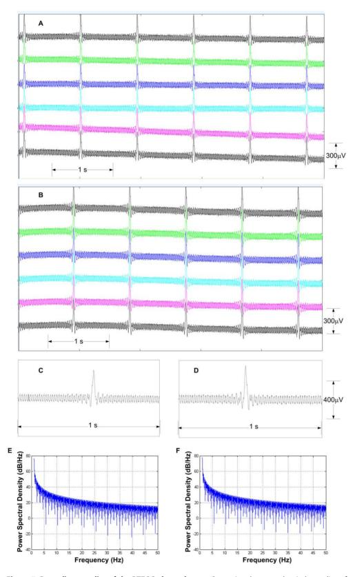
Figure 7. Recordings studies of the PTFOS electrodes set. Comparison between electrical recording of a Sin(x)/x function with amplitude of 300  $\mu$ V of a stainless steel set (**A** and expanded in **C**) and the PTFOS (**B** and expanded in **D**). Comparison between power density spectrum (PSD) of silent (only noise) recording of a stainless steel set (**E**) and the PTFOS (**F**). doi:10.1371/journal.pone.0041187.g007
