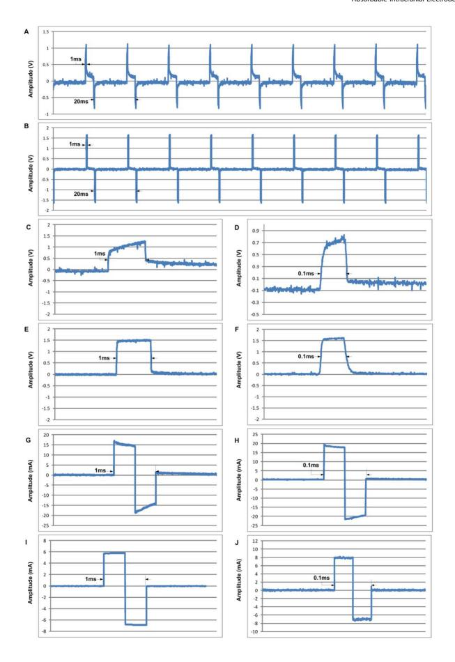
**Figure 8. Stimulation studies of the PTFOS electrodes set.** Comparison between 50 Hz current stimulation with a pulse duration of 1 ms for stainless steel set (**A** and expanded in **C**) and the PTFOS (**B** and expanded in **E**) and 0.1 ms for stainless steel set (**D**) and the PTFOS (**F**). Comparison between 50 Hz voltage stimulation with a pulse duration of 1 ms for stainless steel set (**G**) and the PTFOS (**I**) and 0.1 ms for stainless steel set (**H**) and the PTFOS (**J**).
