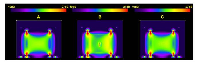
**Figure 4. Results of the electromagnetic simulations.** The  $B_1$  field distribution in a plane inside the head coil and phantom containing: (**A**) no electrodes, (**B**) platinum and (**C**) PTFOS electrodes. The 0dB (red) scale corresponds to a reference value of 3.8  $10^{-7}$  T. doi:10.1371/journal.pone.0041187.g004
