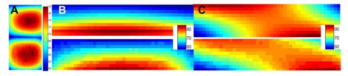
**Figure 5. Validation analysis of the electromagnetic simulations.** Numerical estimation (top) vs. AFI measurements (bottom) of the flip angle in the: (**A**) xy (**B**) xz and (**C**) yz planes. doi:10.1371/journal.pone.0041187.g005
