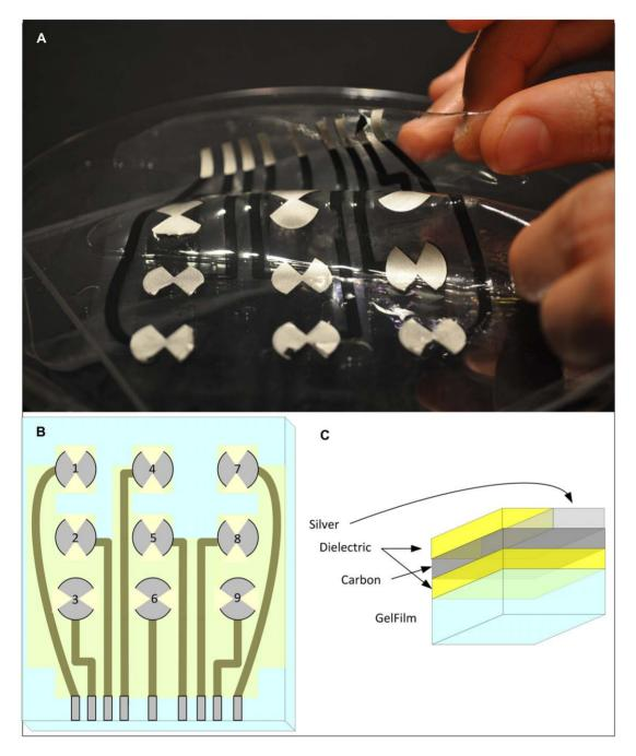
Figure 1. The polymer thick film organic substrate (PTFOS) flexible electrode set. (A) Image, (B) layout and (C) sectional cut of the PTFOS. The 4 layers are made of dielectric, carbon, silver and Gelfilm. doi:10.1371/journal.pone.0041187.g001
